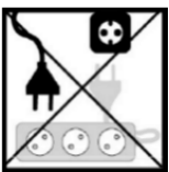
If an extension lead may become overloaded
